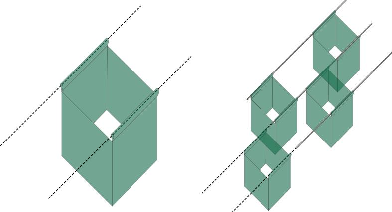
Made from transparent vinyl and strung along cables attached to support columns on the landscape, Peoples Pavilion is a hassle free, durable way to add a bit of color to the neighborhood. Optional addition of wind turbines as seen in the renders, would not only allow this project to not rely on the grid, but potentially give back to the community.
